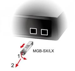
Figure 2-2-5: How to Pull Out the SFP Transceiver
